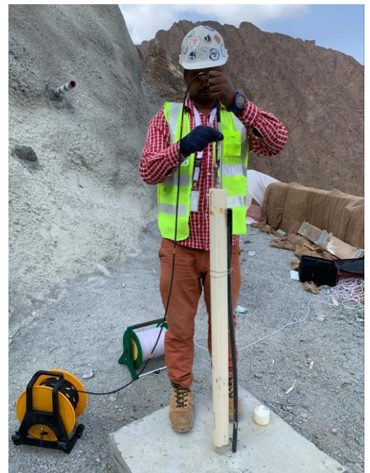
Digital inclinometer monitoring
