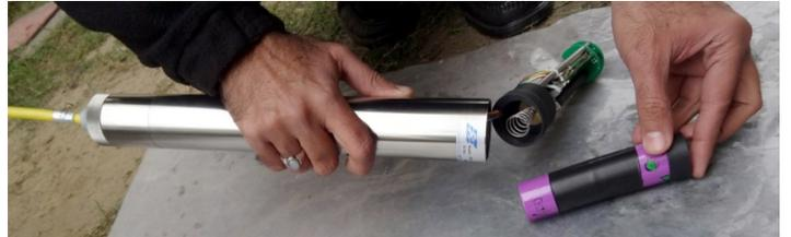
8.11.10 Replace the old assembly of batteries with the new one. Keep positive terminal of batteries upside, covered with cap. Slide back the battery in its place. Refer figure 8-36. Ensure that the batteries are properly set. The top cap will come below the internal threads of the steel housing.
