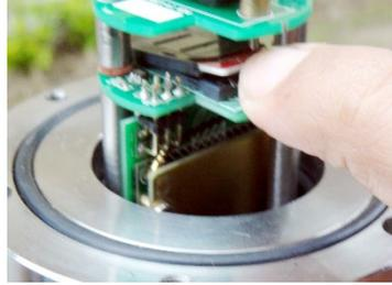
**Figure 8-21: SIM installation**
