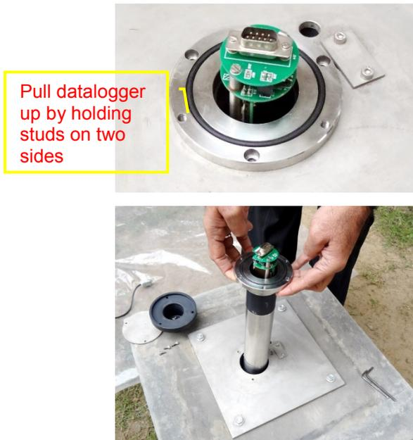
**Figure 8-31: Battery replacement**
