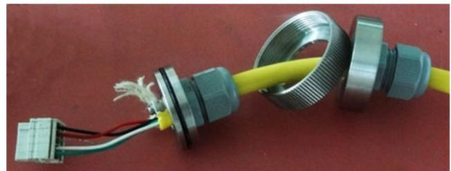
**Figure 8-15: Sensor side cable assembly**
