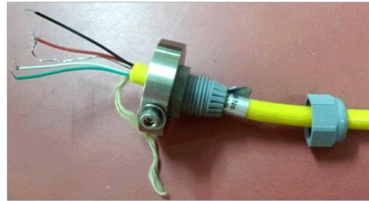
**Figure 8-7: Fixing sensor protector**
