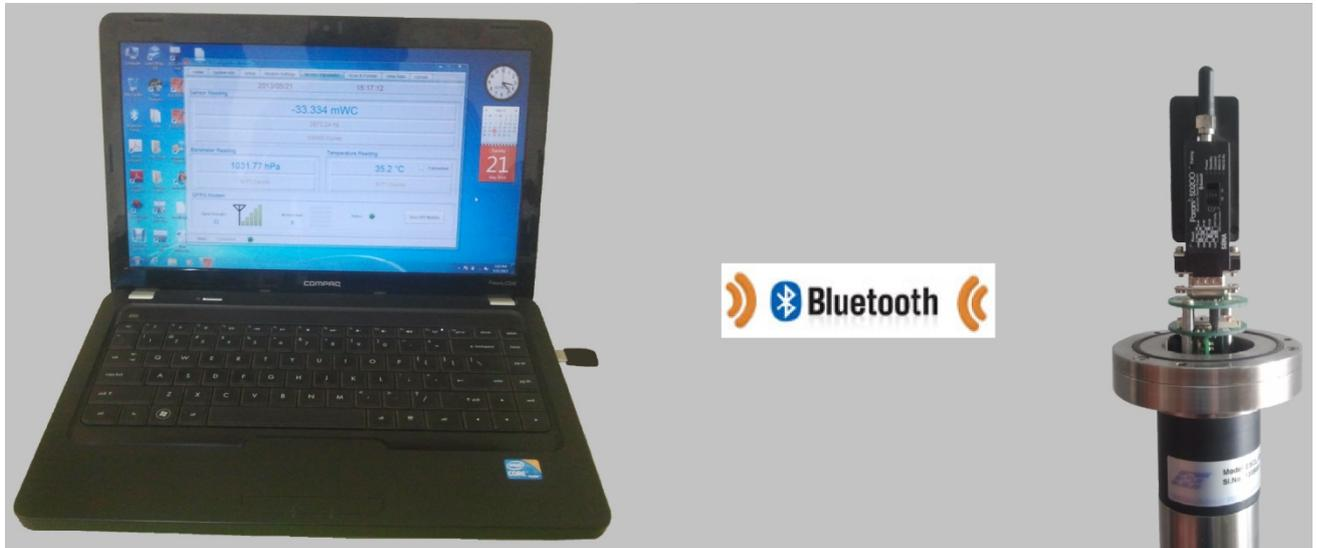
**Figure 7-6: Connecting datalogger using Bluetooth**
