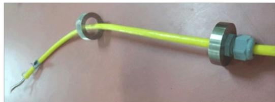
**Figure 8-9: Sliding sensor cable through knurled end cap**
