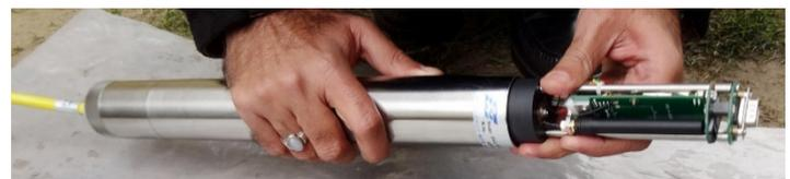
**Figure 8-34: Taking out GSM card assembly**
