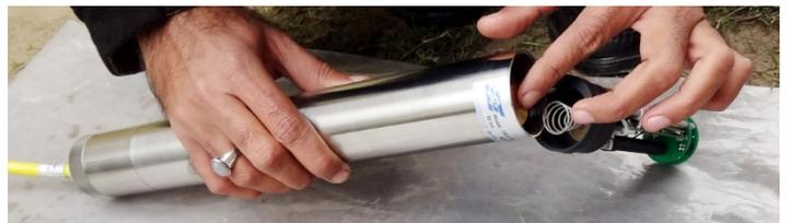
**Figure 8-36: Replacing battery**
