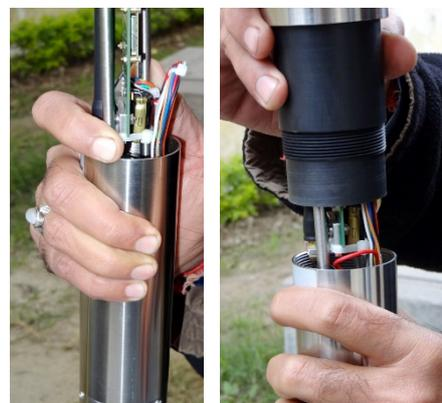
**Figure 8-38: Fixing back the nylon housing**
