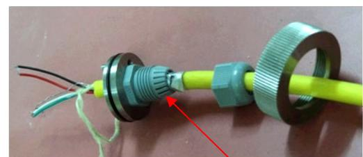
**Figure 8-10: Sliding sensor cable through cable gland holder assembly**
