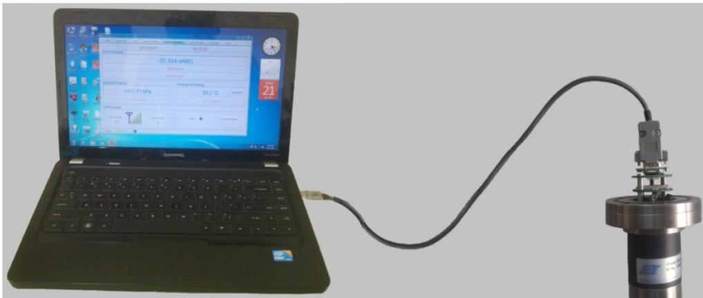
**Figure 7-3: Connecting datalogger using interface cable**
