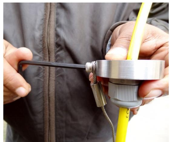
**Figure 9-3: Fixing sensor protector**
