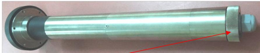
**Figure 8-8: Knurled cap at datalogger lower end**
