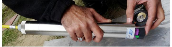
**Figure 8-35: Taking out battery**
