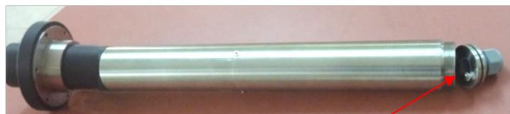
**Figure 8-11: Pulling out cable gland holder assembly**
