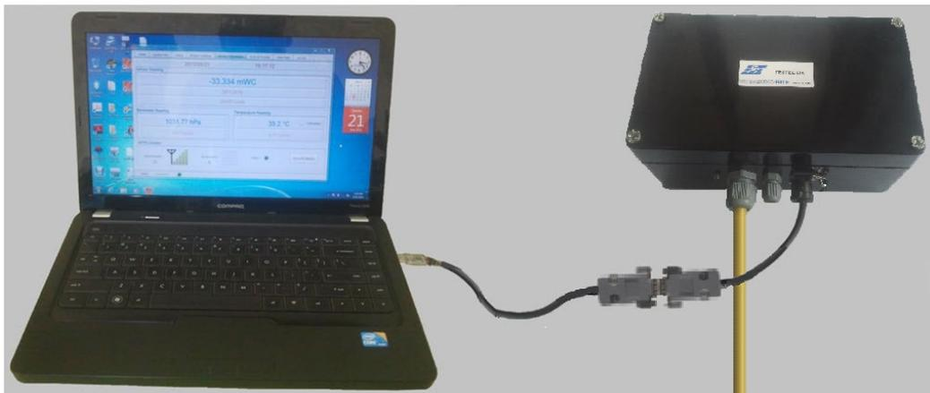
**Figure 7-4: Connecting datalogger using interface cable**
