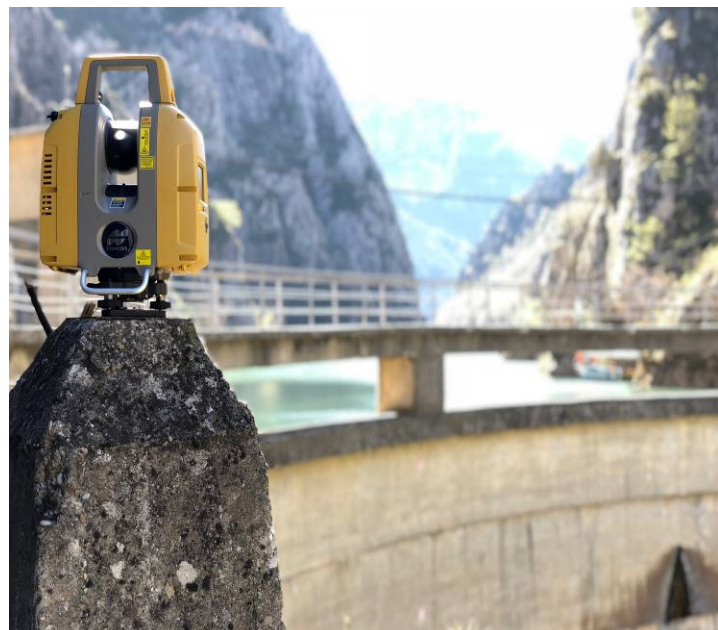
Automatic surveying system (ATS)
