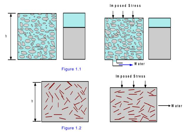
**Surcharging (or pre-loading)** involves placement of fill materials to a level higher than that required for the foundation or embankment, so that consolidation proceeds more quickly. The fill material is removed later on.
