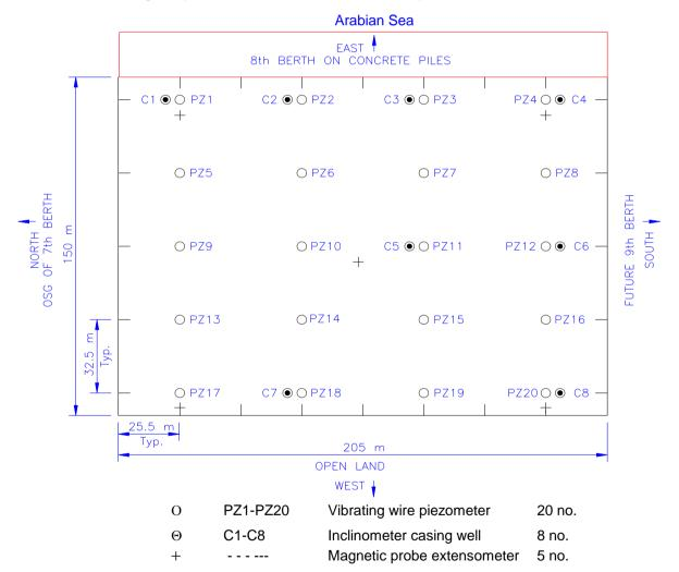
Fig 3.1: General instrumentation layout-OSG area (8<sup>th</sup> cargo berth)
