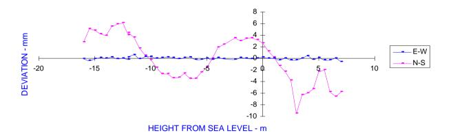
Figure 3.5: Inclinometer readings at bore-hole C1
