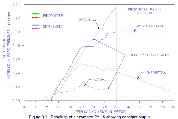
At the location at which the piezometer PZ-15 was installed, the rate of increase of pore water pressure because of pre-loading and the rate of dissipation of water is nearly equal. The amount of pore pressure rise is immediately nullified by quick dissipation of water through the band drains. See figure 3.3 on previous page. Also notice that the settlement is greater than the theoretically estimated value.
