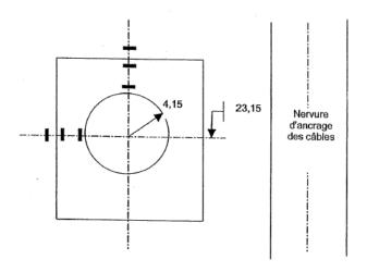
Typical location of strain gages in the equipment hatch
