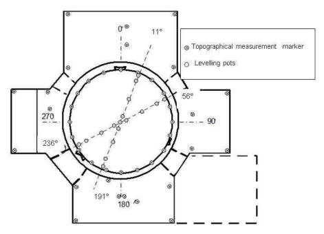
Typical locations of topographical markers and hydraulic settlement system pots in the raft
