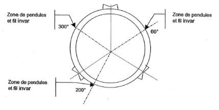
Typical locations for the normal plumb lines with invar wire
